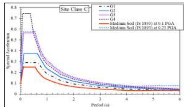
Fig. 2. Typical ADRS for seismic site class C with BIS:1893 (2016) for IGB
