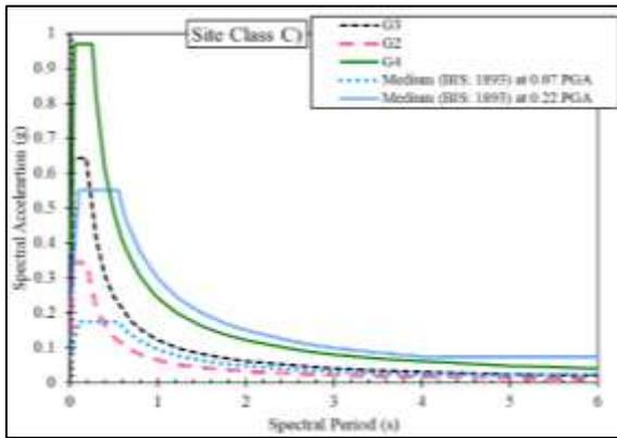
Fig. 3. Typical ADRS for seismic site class C with BIS:1893 (2016) for IGB
